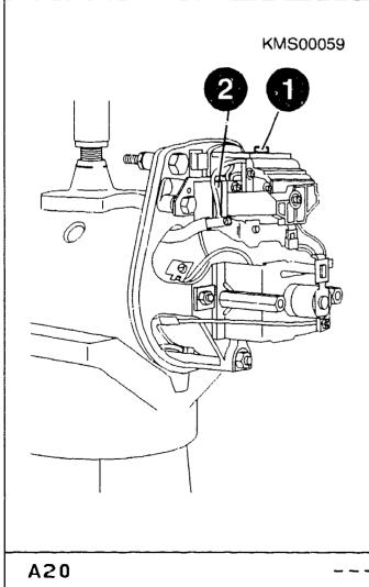
Disassembling control relay and starting-motor solenoid
